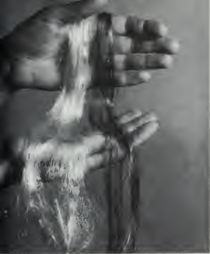
Department chemists made these textile fibers from amylose starch from corn in studies of the utilization of agricultural products.
